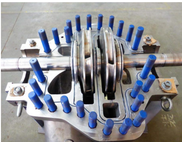
Figure 2 & 3: O-ring sealing at lower pump casing
